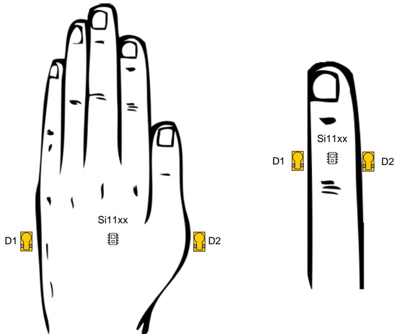
**Figure 1. Ideal Hardware Formations—Hand versus Finger Detection**
