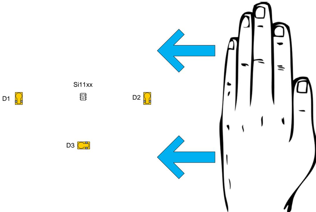
**Figure 5. Swiping Left over a 3-LED System**
